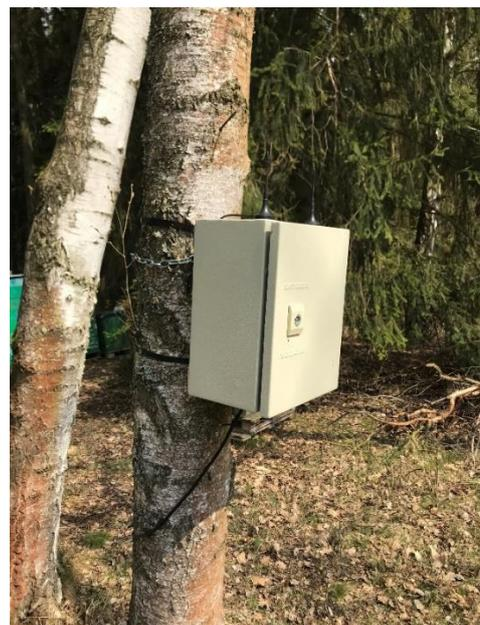
After manual installation of the transmitters and switching on the central unit, it is recommended to monitor on its display whether the central unit has a sufficient GSM signal (value up to 100dbm) and whether its connection with all transmitters has been successful. If so, the installation is complete and after a few minutes the first data in the ProBee online beekeeper's diary appears.
